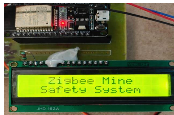
Figure 7. LCD Display Showing Zigbee Mining Safety System Initialization
